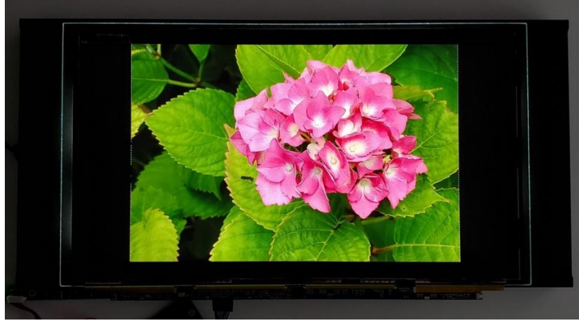
Figure 8. Appearance of prototype display. The OVDs of the prototype display A and B were 689 mm and 344 mm, respectively.
