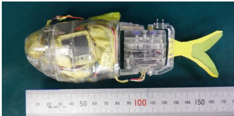
Figure 1. Robotic fish SAPPA (BL = 170 mm).
