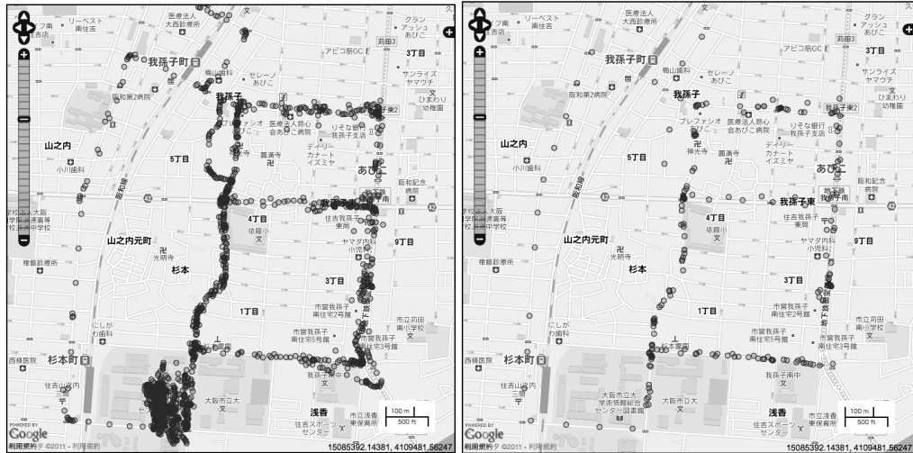
Fig. 6 Result of HDOP based data selection in OpenLayers interface (a) Before data selection (b) HDOP data selection result
