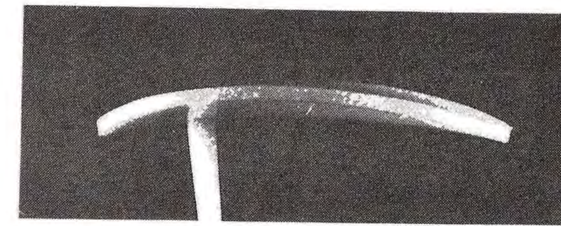
Fig.2-12 Photographs of injection molded test piece. (Circular plate ; Eccentric distance = 25 mm)
