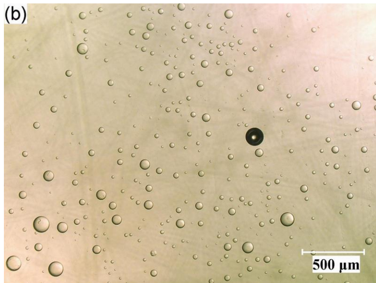
Figure 3–5. Micrographs of oil droplets obtained before nucleation occurred at (a) 75 rpm (coefficient of variation: 1.21) and (b) 200 rpm (coefficient of variation: 0.93).
