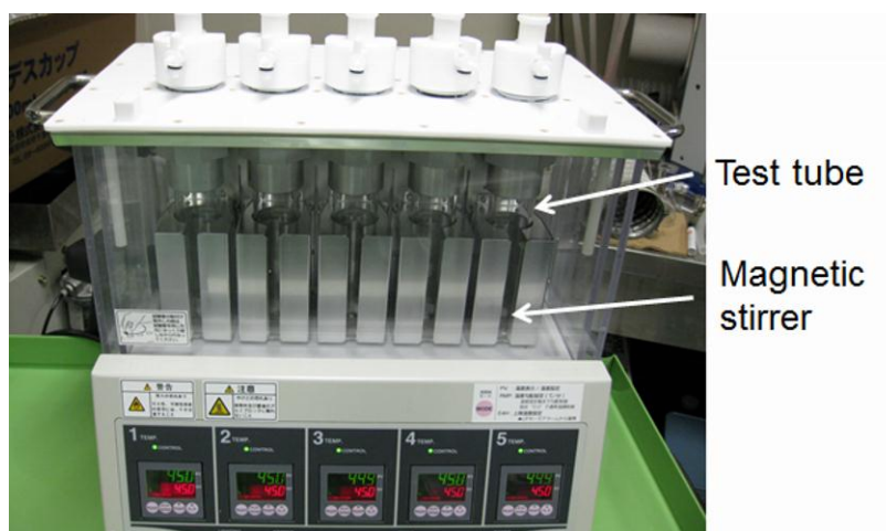
Figure 3-1. ChemiStation TM used in solubility and cloud point measurements.
